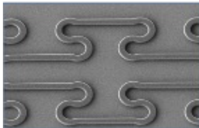
AR-N 4340 Film thickness 2.0 µm Resist structure 4.0 µm
