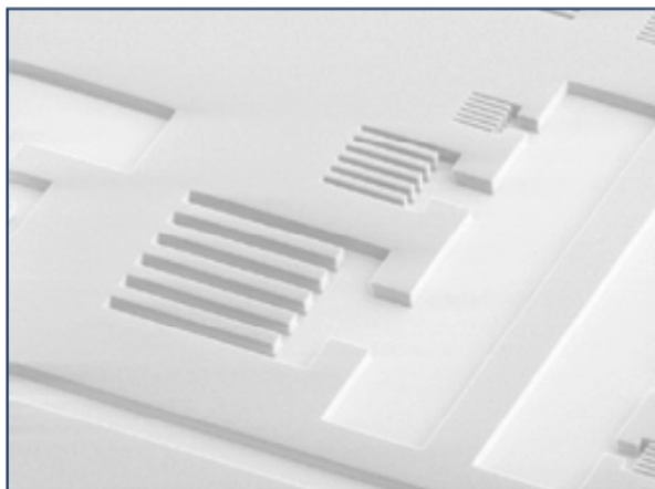
AR-P 6510.17 Film thickness 40 \mu\text{m} , structures up to 5 \mu\text{m}
